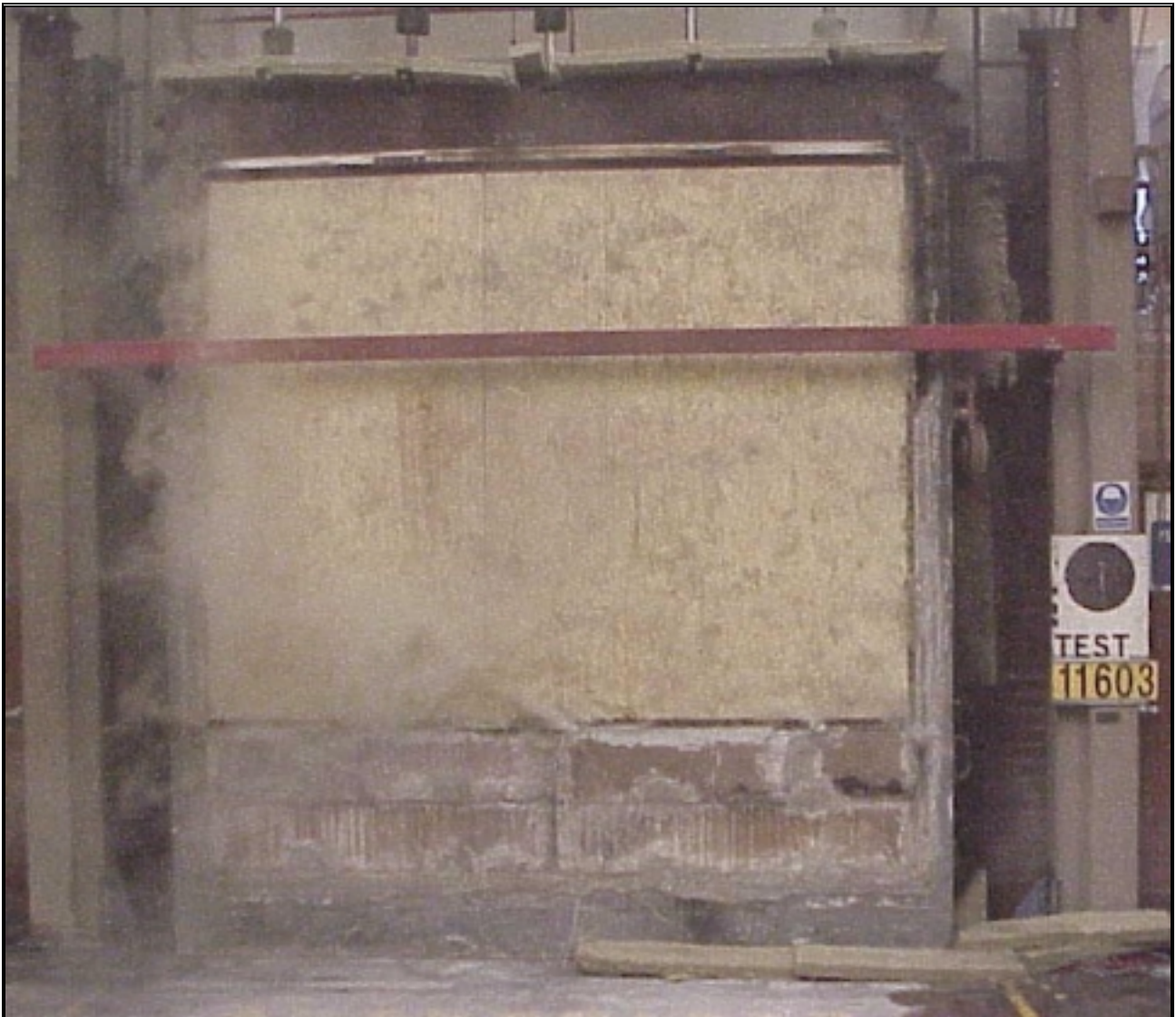
Photo 3. Smoke being emitted from the bottom of the specimen.
